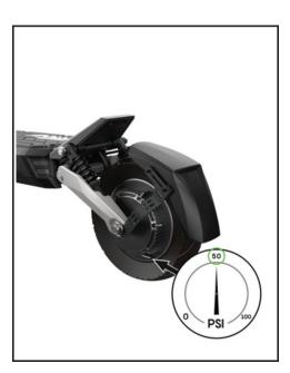
Inflate or deflate the tire as needed until the pressure is 50PSI. Repeat the step with the rear tire.
