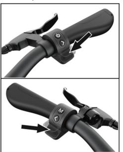
Now test your brakes - Hold the throttle on the right side of your handlebar for 5 seconds, then release and slam both brakes at the same time. The wheel should stop immediately.
