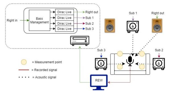
If we further study the measured result in REW, we can see that we have a lot of energy in the lower frequency. We can also see we have no control over this energy with Dirac Live since we have only corrected for each individual speaker.
