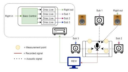
Let's first apply a flat target curve in Bass Control, export the filter and then measures the result in REW. Note, the target curve shows the sum of the three subwoofer and the right front speaker which means that the gain of each subwoofer will be scaled to match the target curve. Raising the lower part of the target curve (below the crossover line) will raise the gain of each subwoofer.
