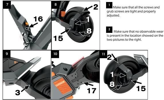
To ensure the longevity of your locking mechanism it is critical to periodically check for any wear and tare that might be happening.
