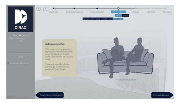
An arrangement can be chosen from the arrangement menu. In the arrangement menu, the home section has three different arrangements: Tightly focused imaging, Focused imaging, and Wide imaging, which provide 9, 13, and 17 measurement points, respectively.
