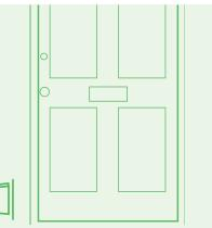
Determine where to place the sensor, remove the wax backing from the adhesive and press firmly for **30 seconds**.
