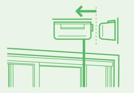
If you have double doors, you can use one sensor to protect both doors. Place the transmitter on one of the doors and the magnet on the other, near the top. Double check to make sure that the indicator arrows are aligned.
