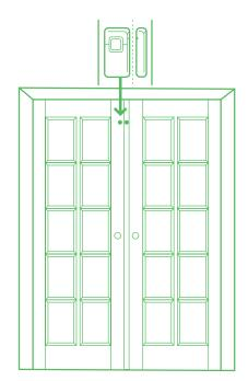
For sliding glass doors that do not align flush with their frame, place the transmitter on the door and place the magnet on the inside of the frame at a *90-degree angle* to the transmitter.
