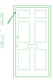
If you have crown molding or any other type of decorative molding, it might be more convenient for you to reverse the setup, with the transmitter on the door and the V magnet on the frame, as shown in the **optional setup**.
