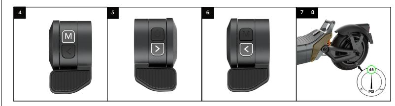
Next, grab an air pump and locate the air valve on the front tire. Remove the safety cap and attach the pump tube to the tire valve. Turn on the air pump and read the PSI measure - the ideal tire pressure for the City is 45PSI.
