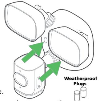
**14** Tighten all knobs and collars by hand to ensure IP66 waterproof protection.
